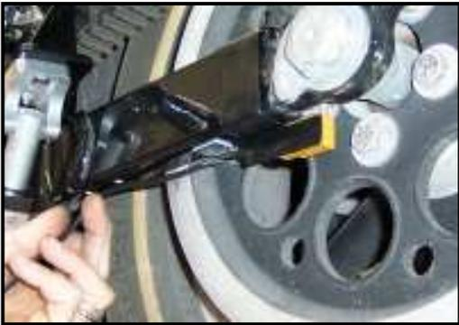
making sure the wire stays snug (not tight). Usually it is best to join the wire to the leads from the actuator, leaving some slack, to allow movement on the actuator, as well as the swing-arm. Then route these wires into the area under the left side cover, where they will be connected again to their mating plugs. Extreme care must be used here to make sure everything clears the belt and is secure. On some bikes removal of the lower belt guard may be required.
