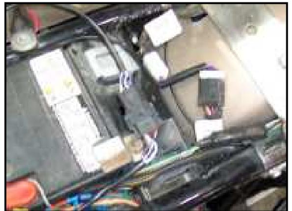
Don't tie down the wires just yet but if you have all the plugs connected, we can do a quick test of the system. There are 2 things we want to check here. We want to make sure the controls work, and we want to check the light on the proximity sensor is functioning.
