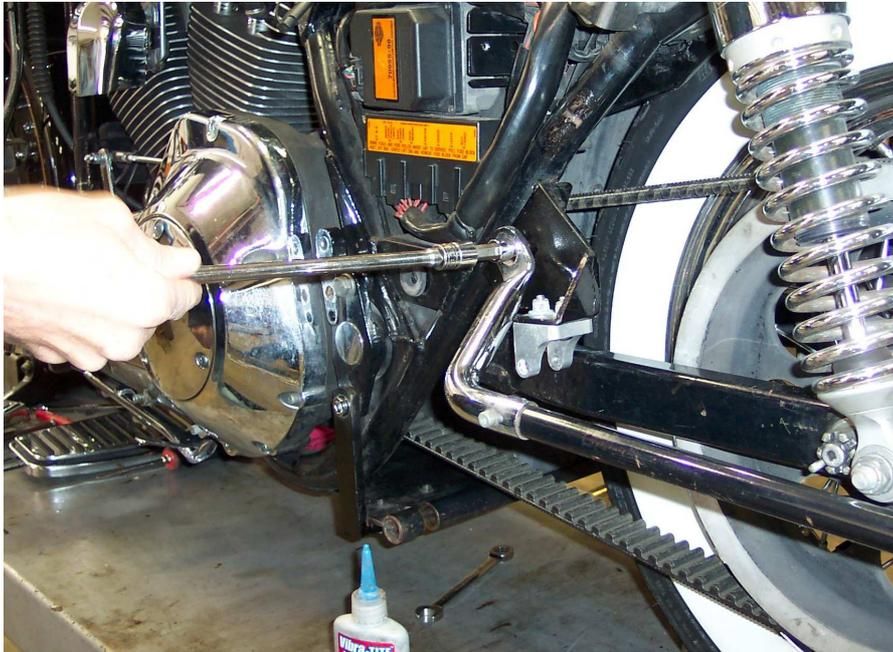
Attached to this bracket is the upper actuator mount (brushed aluminum) with the upper actuator axle. This mount is left intentionally loose and will be tightened during the alignment of the actuator.
